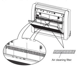
Install the Air filter and close the Intake Grille.
