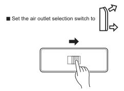
Air blows out automatically from the upper and lower air outlets as shown in the table below.
